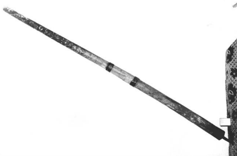
Fig. 14. Sleds braking stick kauripo. Nanai of Kondon village. Photo by author, 1998. .
